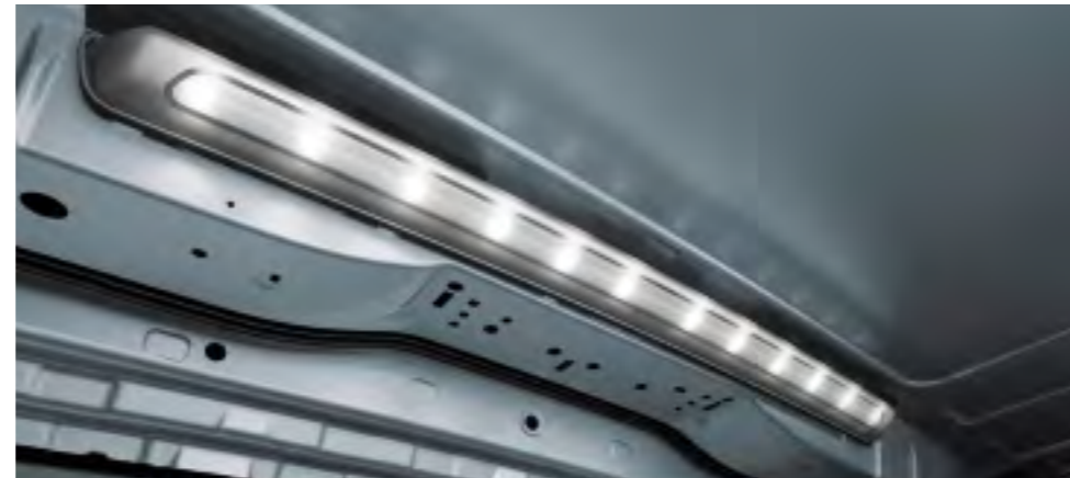
The LED light strip at the top in the rear illuminates the load compartment so that there are minimum shadows and thus improves orientation when loading and unloading. Optional.
