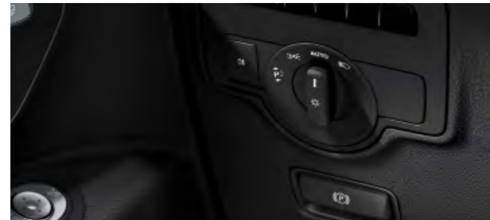
The automatic driving lights function switches the driving lights on or off, depending on light conditions.
