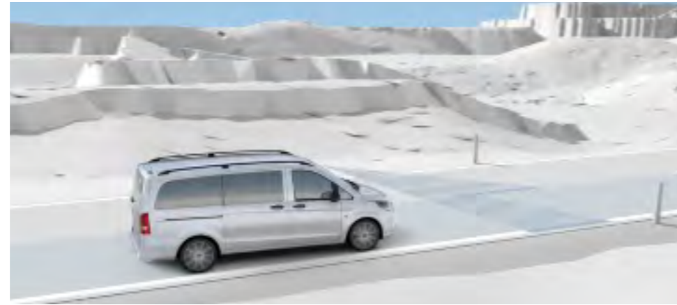
The Blind Spot Assist (7) (visual and audible warning) and Lane Keeping Assist (haptic and audible warnings) can help the driver stay in lane or change lanes on multi-lane roads.
