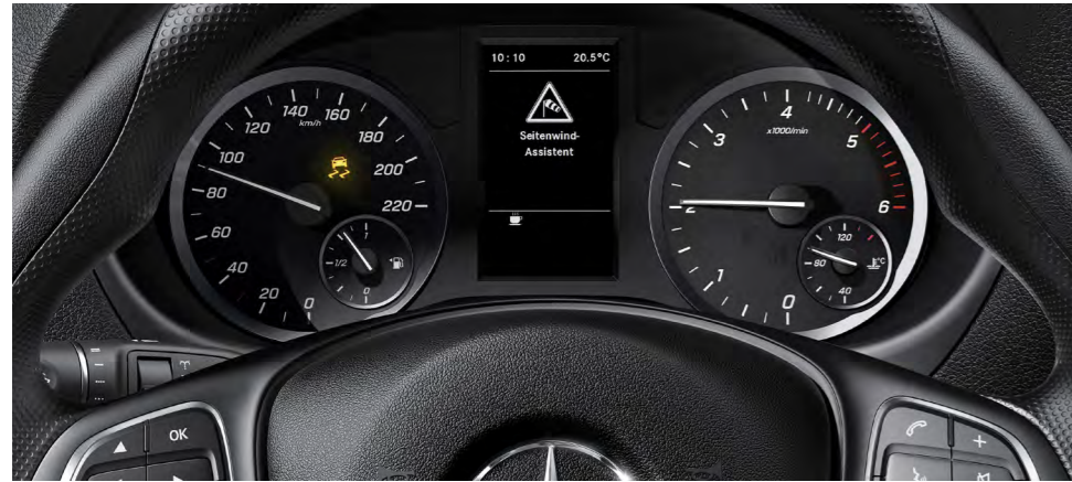
Crosswind Assist can detect track offset caused by strong crosswind gusts in good time and help the driver to stay in lane. A sudden track offset of the vehicle can cause inappropriate steering reactions on the part of the driver.
