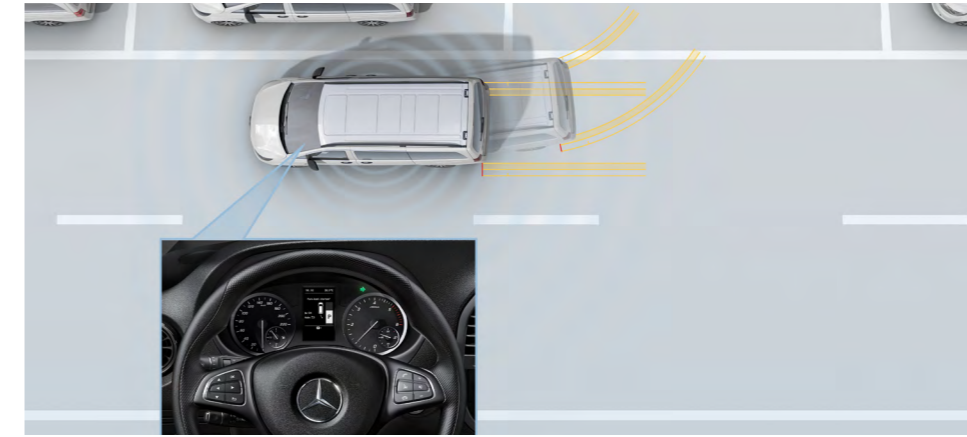
The Active Parking Assist feature can detect parking spaces and supports with active steering interventions when parking in longitudinal or lateral parking spaces. Optional on all 111 models.
