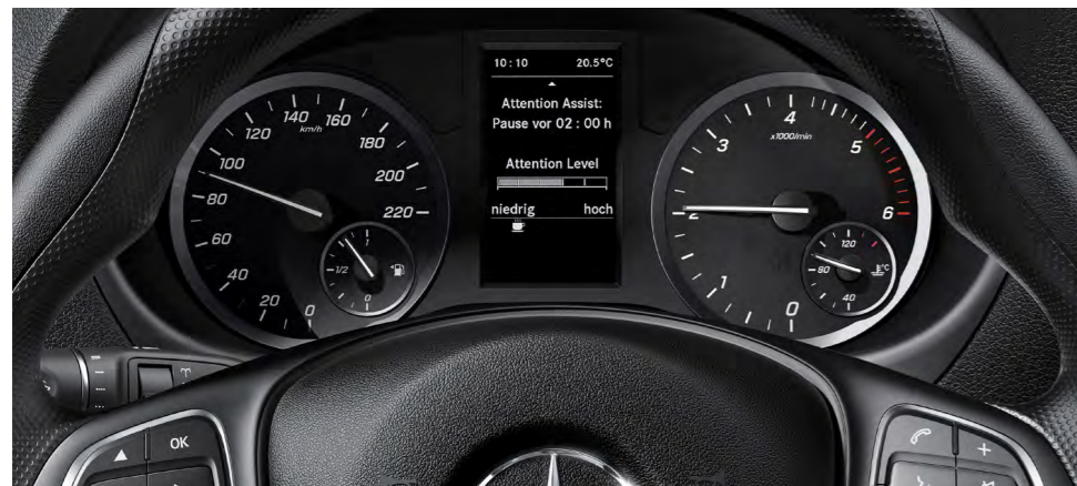
The ATTENTION ASSIST system can help to avoid momentary nodding off and therefore provides you with increased safety, in particular when driving at night and on long journeys. The system provides you with a visual and audible warning if it identifies typical signs of fatigue or attention lapse, and suggests taking a break.
