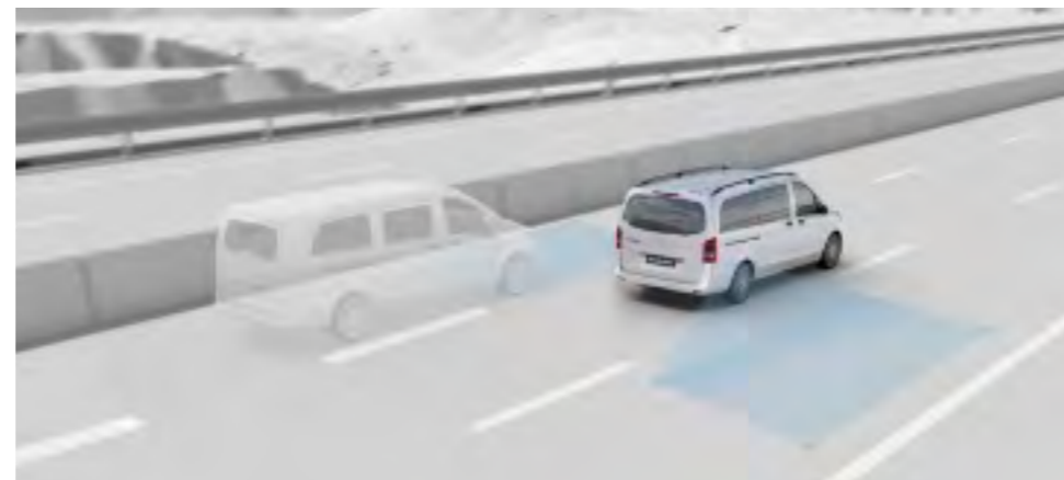
The Blind Spot Assist (7) function can help prevent accidents when changing lanes, for example on motorways.
