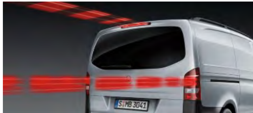
The adaptive brake lights with their conspicuous flashing assist to reduce the reaction time of the drivers of following vehicles and therefore prevent rear-end collisions.
