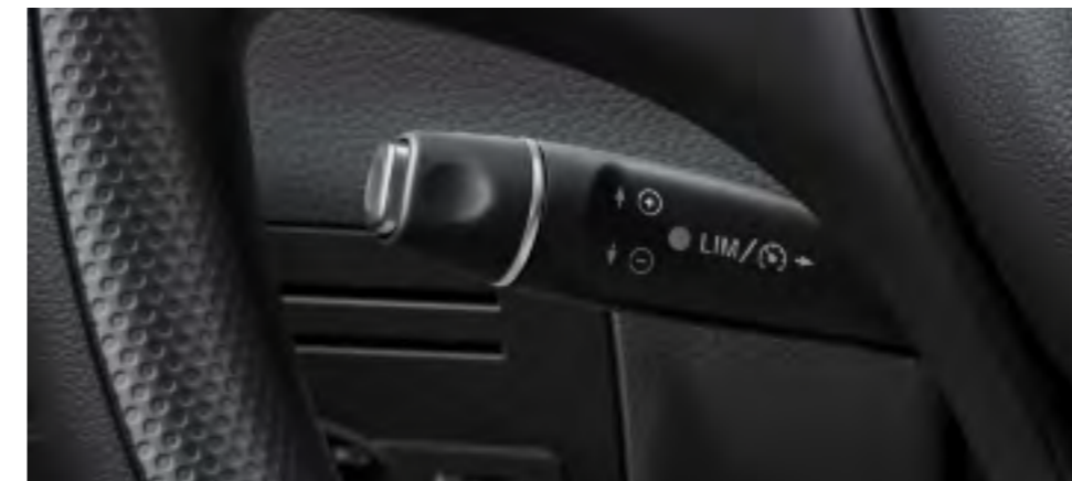
The cruise control system with Limiter maintains a pre-selected speed and thereby makes driving more relaxed and more economical – especially on long distances. Standard on 111 models.
